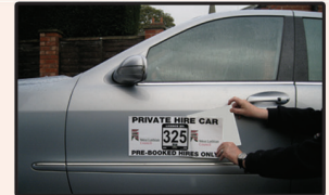
Slowly pull down backing sheet and smooth down from hinge.
