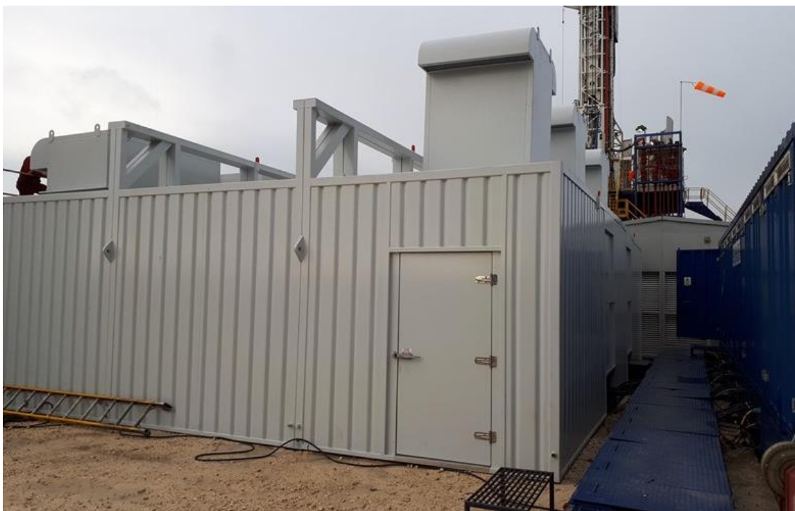
Figure 6.3: Example mud pump housing
