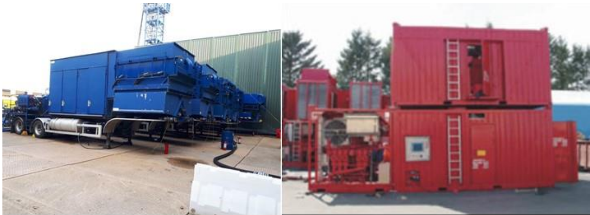
Figure 6.9: Example frac pump enclosure
